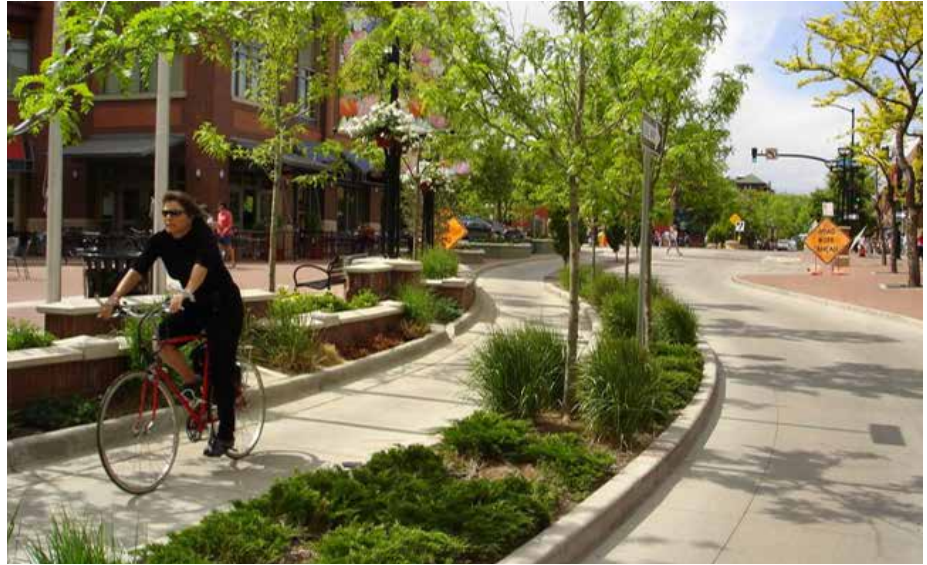
Use striping, vertical separation elements, or other design features to provide separation between bikes and major vehicular routes.
