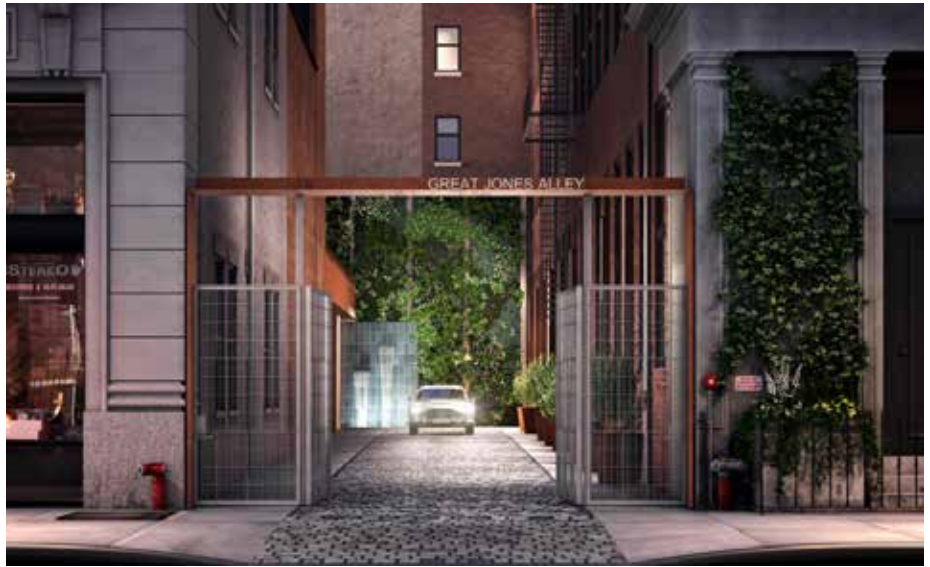
Clearly identify vehicle access to raise awareness of ingress/egress with distinguishing design elements such as paving materials, colors, or patterns and signs.
