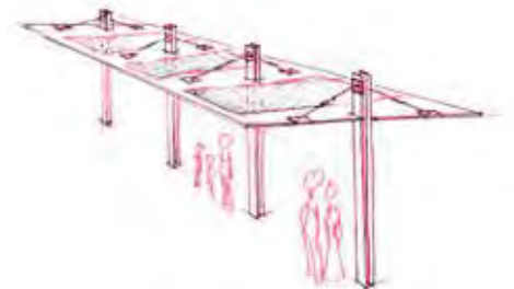
A walkway shade structure inspired by industrial materials. A flat metal canopy is supported by steel I-beams and turnbuckle systems.
