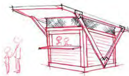
A concession/information stand inspired by the materiality and construction techniques in the pens area. A simple shed roof is supported by a wood beam structure. Plank siding could utilize reclaimed wood from historic pens.
